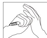
The body is made of space grade aluminum with precision machining and Mil - Spec Type III hard anodizing process, with its tip topped with Tungsten steel, which hardness can reach at HRA 89 to 95, which quality makes sure it can be used for glass breaking in emergency situations and durable usage.
